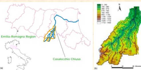
Figure 2: (a) The upper Reno river basin (~1000 km<sup>2</sup>) in the Emilia-Romagna Region, northern Italy. The discharge forecasts are evaluated at Casalecchio Chiusa, the closure section. (b) The Digital Elevation Model (DEM) and the sub-catchments defined in the implementation of HEC-HMS model for the Reno river basin.
